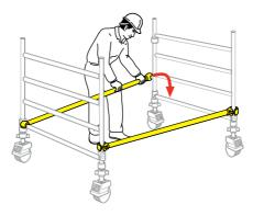
**4** Fit 2 additional end frames and check the frame interlock clips are engaged. Fit 2 diagonal braces (blue) in opposing directions, between the 2nd and the 6th rungs. Ensure the frames are vertical and level by checking with a spirit level and setting the adjustable legs as required.
