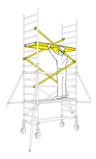
**5** Climb up the inside of the tower and from the protected position of the trapdoor, fit horizontal braces as guardrails, on both sides, to the 14th and 16th rungs (2 and 4 rungs above the platform, in that order).
