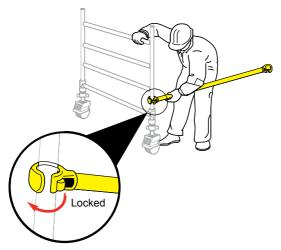
**3** Position the second end frame as shown and fit the other end of the horizontal brace on to the vertical, just above the bottom rung. Fit a second horizontal brace between the bottom rungs on the other side of the frames to square the tower.
