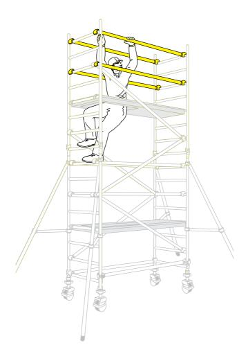
6 Continue the procedure until the required working height is reached, adding additional pairs of end frames, diagonal braces and fitting trapdoor platforms, as shown on previous steps. At every platform level, add horizontal braces as guardrails at 2 and 4 rungs above the platform (in that order) on both sides of the platform. (as shown in Step 5)
