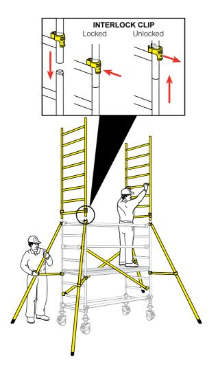
**4** Fit 2 pairs of diagonal braces in opposing directions between the 6th and 10th rungs and the 10th and 14th rungs. Locate a trapdoor deck on the 12th rung.
