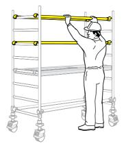
**3** Fit 2 diagonal braces (blue) in opposing directions between the 2nd and 6th rungs. Ensure the frames are vertical and level by checking with a spirit level and setting the adjustable legs as necessary. Fit the next pair of end frames and check the frame interlock clips are engaged. Fit stabilisers (see notes on page 30).
