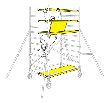
**6** Fit the next pair of diagonal braces in opposing directions between the 6th and 10th rungs add 2 additional end frames.
