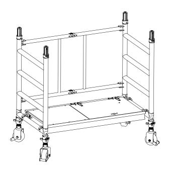
Fit the folding toe board set to the trapdoor deck.
