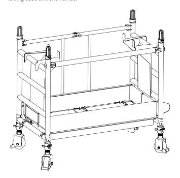
Place the camlock frames, three at either end within the trolley. Ensure the diagonal struts of the camlock frames fit between the arms of the assembly brackets.
