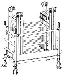
Add the final trapdoor deck in front of the 1m end frames. Fit the four SP4 stabilisers in front of the trapdoor deck. The trolley unit is now complete.
