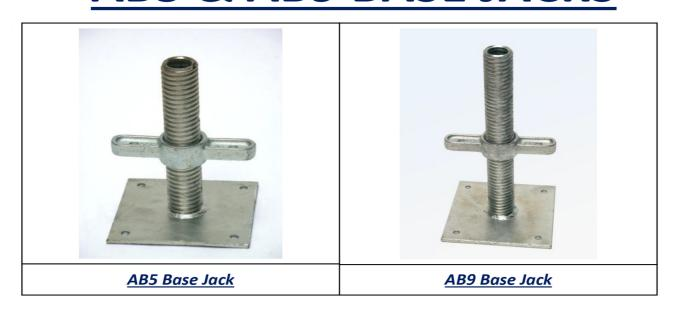
Delta have been renowned manufacturers of Scaffold Base Jacks for many years and supply several types, all made using a "roll threading" technique which doesn't cut material away and therefore maintains a high level of strength. Delta Base Jacks are compatible with all system scaffolds.
